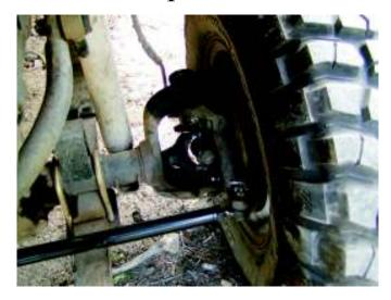
Finding front axle and u-joint damage, the search for repair parts came up short and
