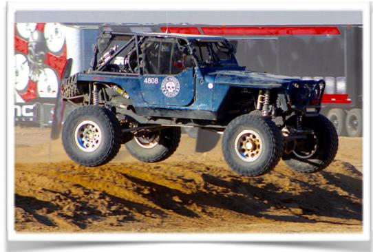
My jeep is set up well for rock crawling but it is far from a desert racer. In order to prepare the jeep for the race I needed to get the following accomplished, either for better performance or to pass the stringent safety inspection: new driveshafts, replaced front and rear ring and pinion's, installed a spool in the rear axle and new grizzly locker in front axle, new atlas 3.8 t case, front axle
